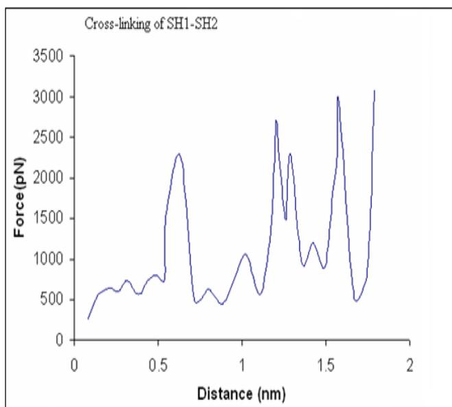
**Fig. 1C:** Force-distance curve of SH1-SH2 crosslinking with nucleotide binding site closed. Force constraints with a spring constant of 16.7 N/m were used to crosslink the reactive cysteines by changing a distance of 0.1nm decrements followed by energy minimization. The force-distance curve was determined by calculating the difference between the actual distance and the target distance after each energy minimization using the spring constant.
